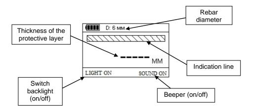
When approaching to reinforcement, the length of the indication line decreases and the frequency of the audio signal increases.
